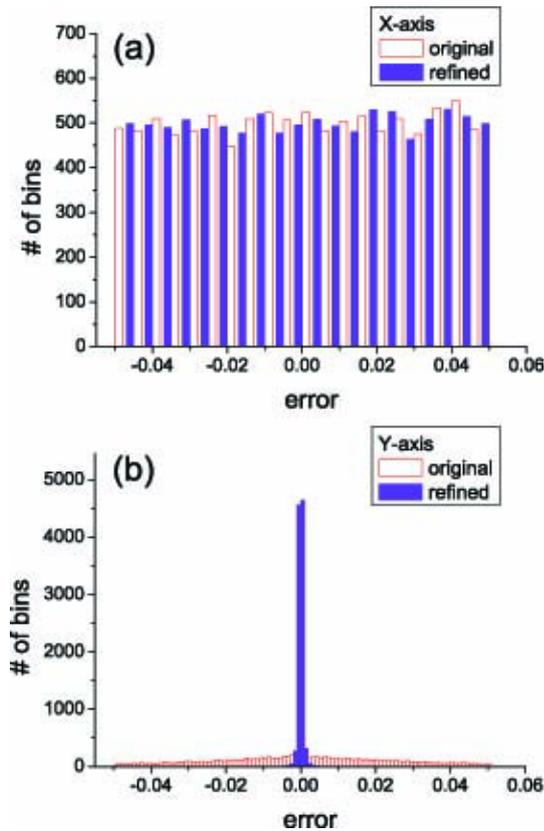
Fig. 3. Directionality of noise reduction in the generalized baker's map. The noise remains at the same level along the  $x$ -axis (stable direction), while it shrinks to zero, as expected, along the  $y$ -axis (unstable direction).
